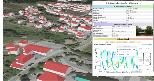
Figure 3: Web 3D visualization with a dashboard showing energy production from a solar panel and environmental data Wüstenrot, Germany
